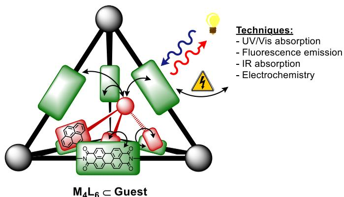
**Figure 3** Host–guest system indicating pyrene-PBI interactions and through-space wall effects. Red sphere = spectroscopic handle (*i.e.* P-X, X = O, BH<sub>3</sub>).
