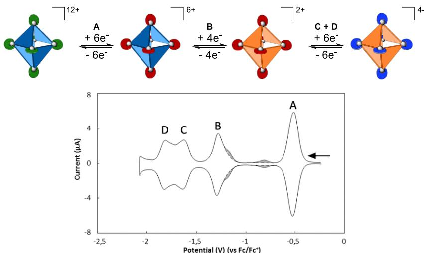
**Figure 4** Convolution plot of BIAN-Pt cage in DCM demonstrating full reversibility of the supramolecular assembly. Individual reduction processes A-D are labeled above the waves.
