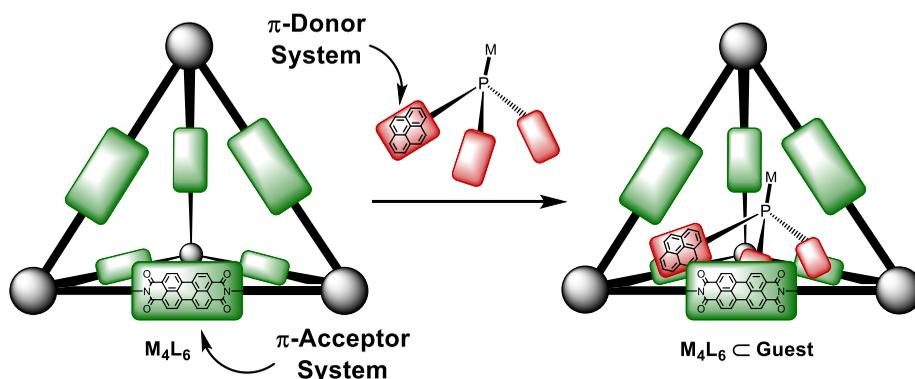
**Figure 2** Schematic illustration of the concept. A cage with electron-poor  $\pi$ -systems (acceptor) as walls binds a (metal)phosphine containing multiple electron-rich  $\pi$ -systems (donor).
